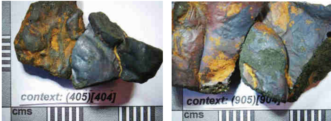
Plate 1 Tap slag from context (405) [404] in Trench 4 (left) and Tap slag from context (905) [904] in Trench 9 (right)
